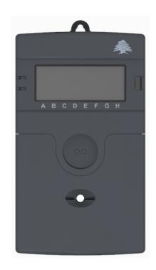
Rated for 220V – 50Hz, and with the ability to measure currents for up to 100 Amps, this meter contains an independent measuring element, thus allowing consumed energy to be measured on both line and neutral phases. All while providing the user with the ability to visualize various accessible parameters on an LCD screen located on top of the meter with couple of led indicators.
